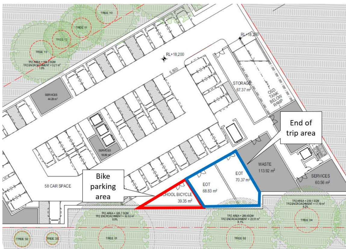
Figure 13 Bicycle parking and end of trip facilities
